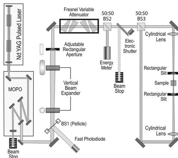
**Figure 2.** Schematic diagram of the laser apparatus used for measuring the photostability of the light-transducing proteins. The relative shape of the laser beam is shown using dotted lines next to the relevant optical component (see Supporting Information for experimental details).
